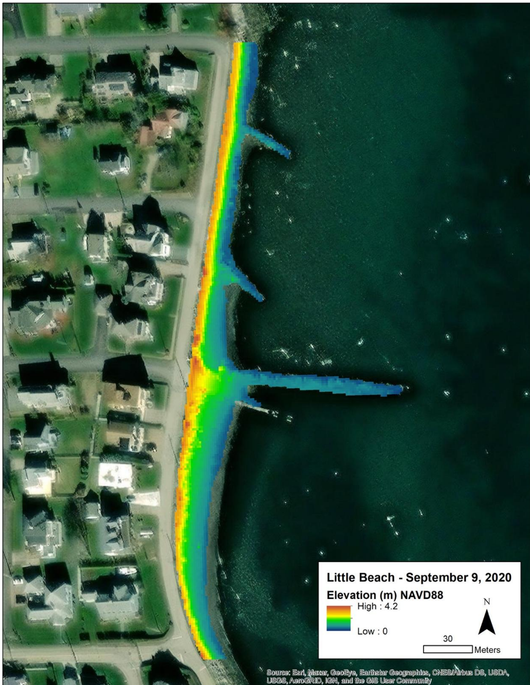
Figure 2-8. Interpolated Digital Elevation Model of Little Beach berm, September 9, 2020. Final DEM representing only beach elevations along Little Beach. All non-bare earth points were removed before producing the 1x1 meter gridded surface.
