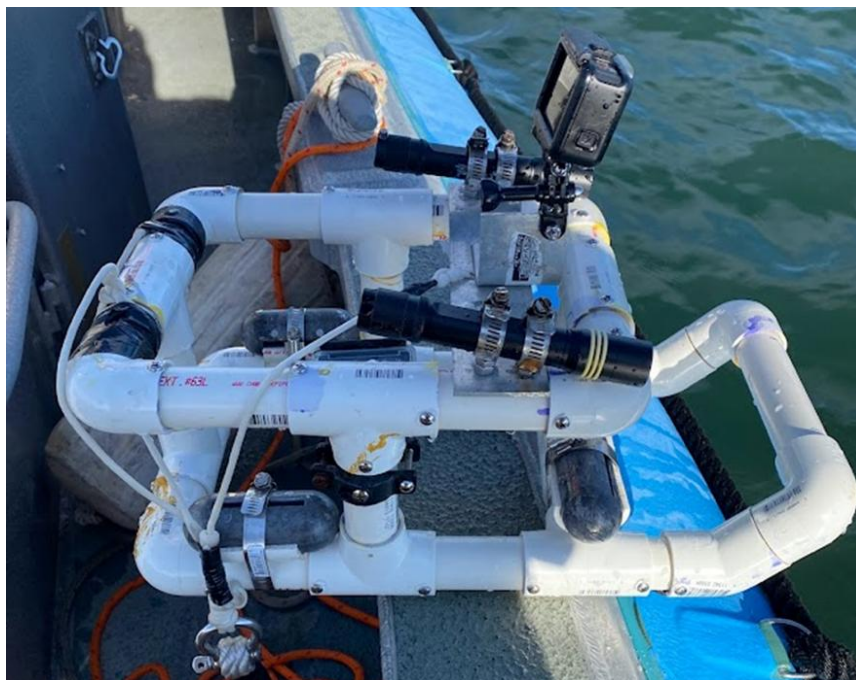
Figure 3-3: Custom built PVC Camera sled used to record underwater video imagery along the drift shown in Figure 3-6.
