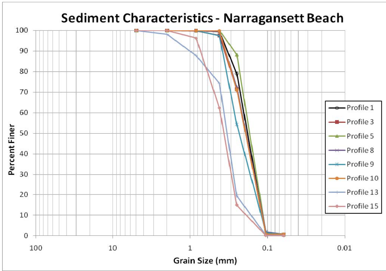
Figure 4-19. Grain Size in Narragansett Beach from Narragansett Town Beach Replenishment Feasibility Project
